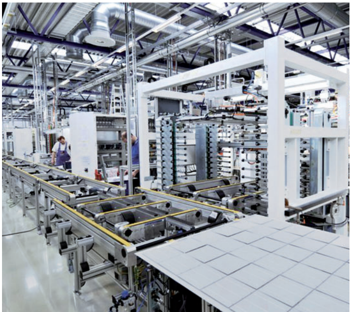
▲ TS 2 pv linking system for solar panel production
