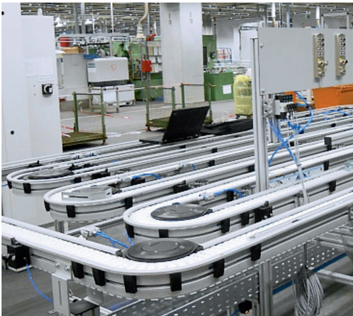
▲ VarioFlow 90 linking system for automotive gearbox machining
